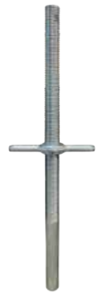
PSV-133N 1-7/8" X 36" Shoring Screw Jack WT. 10.20 LBS
